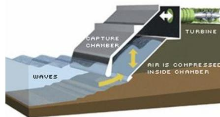
Figure 14 – Example of Active breakwaters<sup>15</sup>
