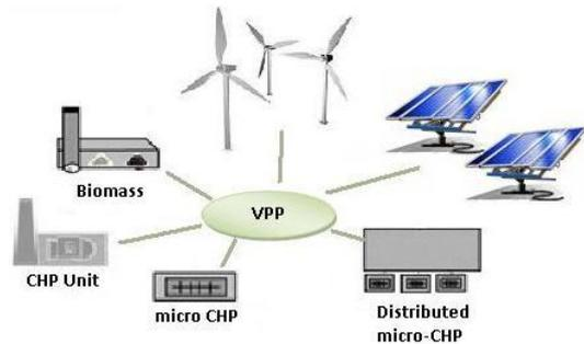
Figure 3 – Diagram for a Virtual Power Plant (VPP)
