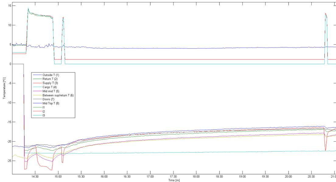
Figure 5: Behavior when setpoint is changed from  $-22^{\circ}\text{C}$  to  $-17^{\circ}\text{C}$
